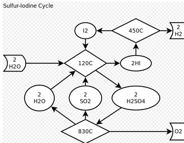
At the bottom of the diagram above,  $\text{H}_2\text{SO}_4$  decomposes into  $\text{H}_2\text{O}$ , oxygen and sulfur dioxide. The reaction is:
